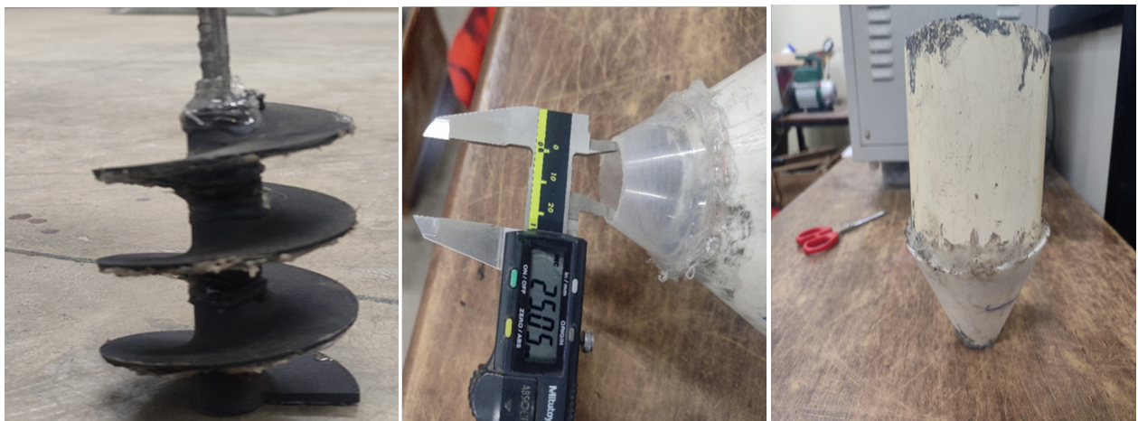
Figure 9: Hopper (Right), Nozzle (Middle) 25mm, screw feeder (Left)
