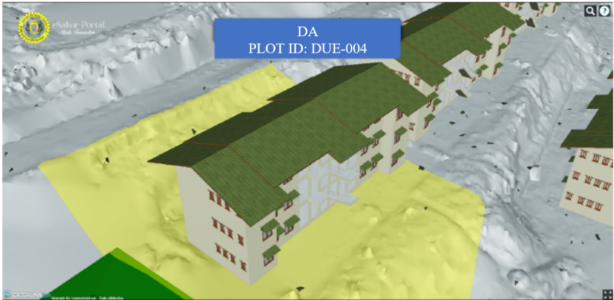
Figure 7: Integration of the 3D building, DTM and 2D plot boundary in CaesiumJS
