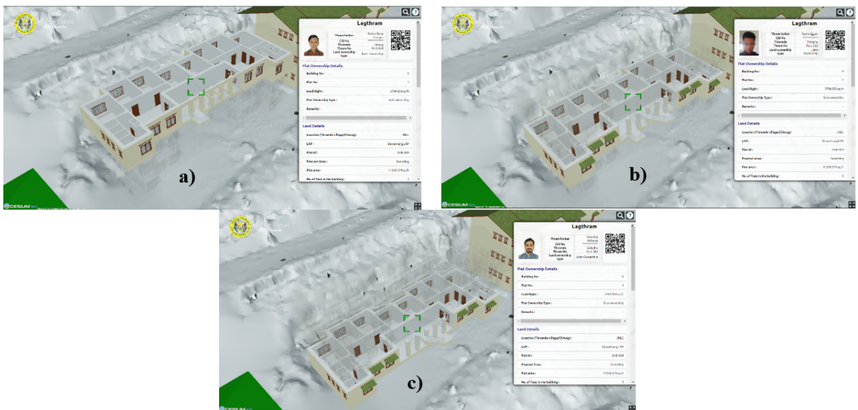
Figure 8: 3D Cadastral Strata information of Duekhor Khangzang-A building of different flat owners for a) second floor b) first floor and c) ground floor
