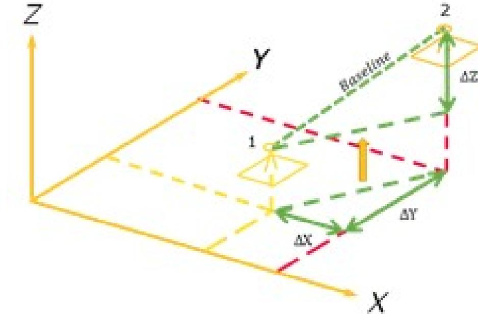
Figure 4: Calculating baselines using Pythagoras' Theorem
