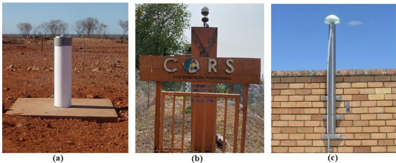
Figure 1: CORS monuments: (a) Tier 1 concrete pillar, (b) Tier 2 concrete pillar from Deothang CORS (DTNG), and (c) Tier 3 wall monument.
