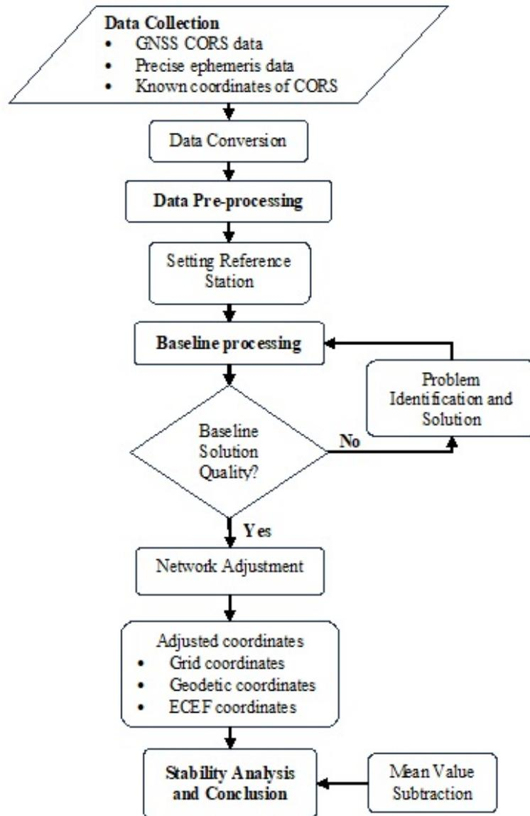
Figure 3: Flowchart of CORSNet data processing and stability analysis
