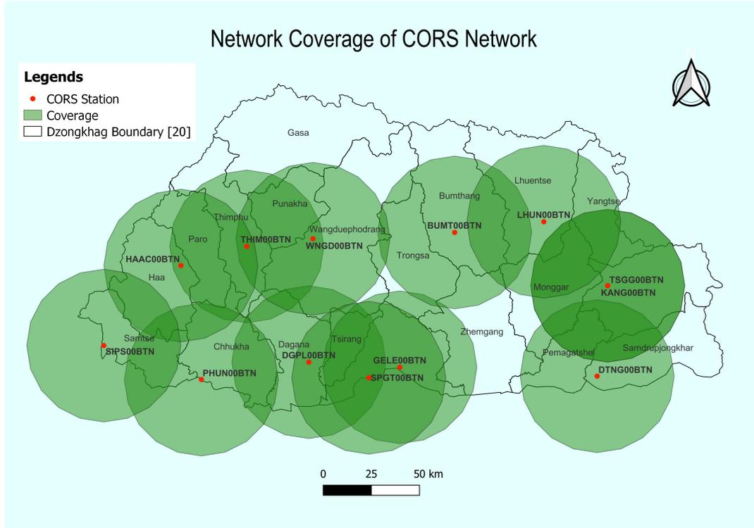
Figure 2: The network coverage of the DRUK CORSNet Stations as of August 1, 2023
